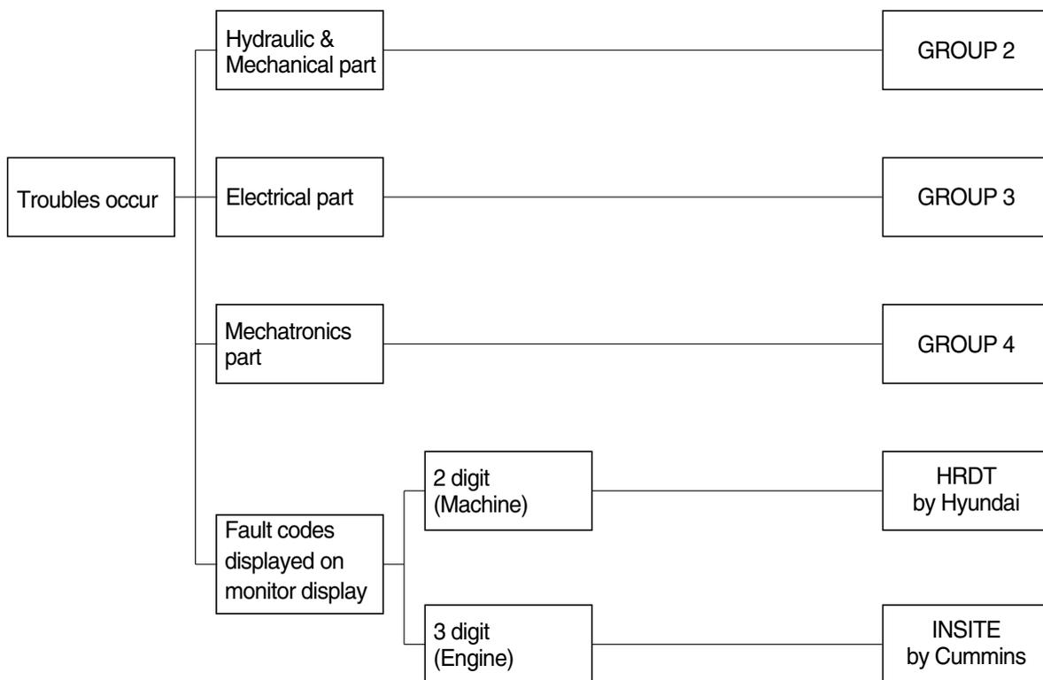
※ If fault codes (2 or 3 digits) are displayed on the monitor, please contact Hyundai or Cummins.
