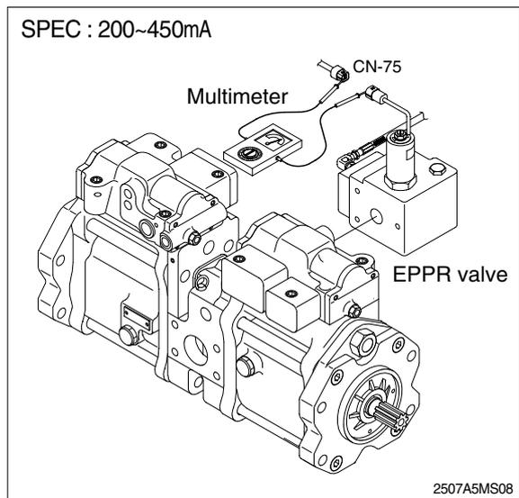
(2) **Test 5** : Check pressure at EPPR valve at H-mode
